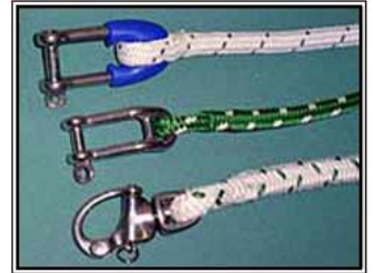
The construction of double-braid line like that shown here makes it uniquely suited to splicing for halyards or other purposes.
