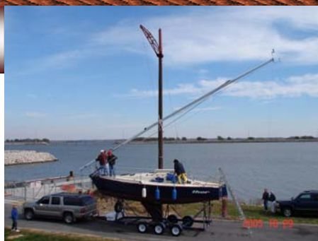
THOR's mast is easy to get down thanks to the new gin pole! (photo by Stephen Hollingsworth)
